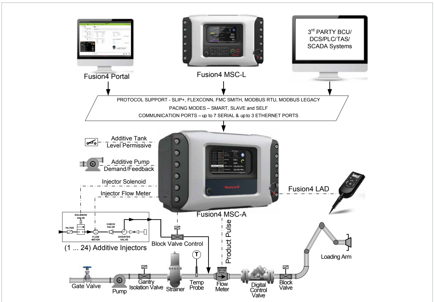
Pictorial representation showing a basic setup of the additive controller. Additional interfaces might be needed, depending on site requirements.
