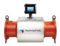
The Smith Meter® Ultra 4c liquid flowmeter is a fourpath ultrasonic meter for custody transfer measurement of petroleum products. The meter provides highly accurate measurement over a range of light to medium crude oils and refined products using an exclusive four-path design.
