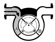
Unmeasured liquid (represented by the dark area in the drawing below) is shown entering the meter, causing the meter's rotor and blades to turn counter-clockwise. Blades A and B are fully extended, forming the measuring chamber; the opposite ends of blades are retracted and flush with the rotor.
