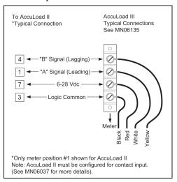
For quadrature (two channel) meter installations with reverse flow direction, refer to the following wiring diagram and reverse white and yellow wire connections. Yellow wire becomes the "A" signal and white wire becomes the "B" signal.
