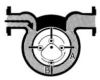
One-eighth of a revolution later, the measured liquid moves out of the meter. Blade A retracts on the outlet side and starts to extend on the inlet side to form another measuring chamber. A second measuring chamber forms between blades B and A as the rotor rotates around the cam.
