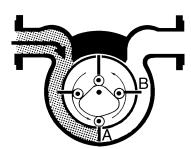
In the drawing below, the rotor and blades have made a one-eighth revolution. Blade A is fully extended; blade B is partially drawn back; and the opposite end of blade B is starting to extend.
