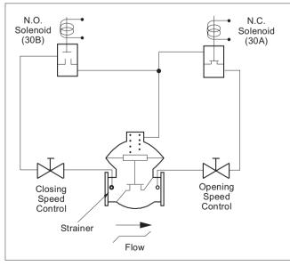
Figure 1. Model 210 Valve Schematic
