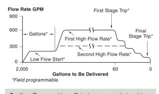
**Caution:** There must be sufficient pump capacity to achieve the flow rate set into the AccuLoad or microLoad or the valve may close slowly resulting in a spill.
