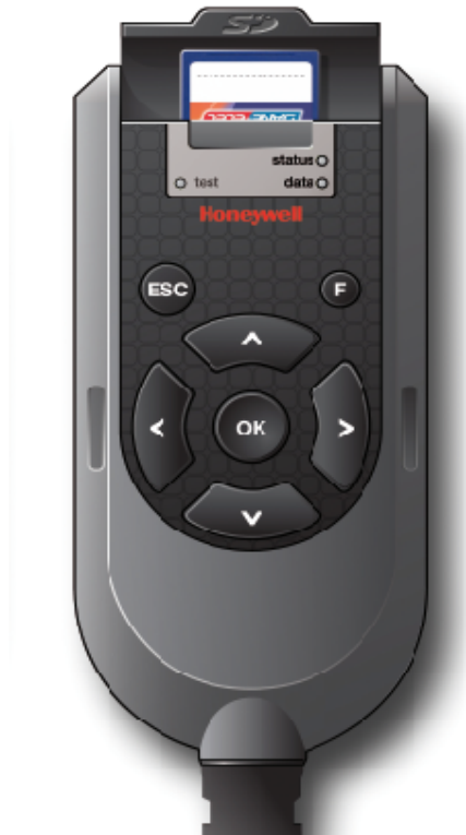
FIGURE 5-6 SD card location in LAD (lid opened)
