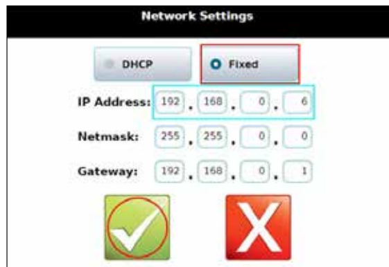
Figure 158: Changing the Internal IP Address (SA Model)—Network Settings
