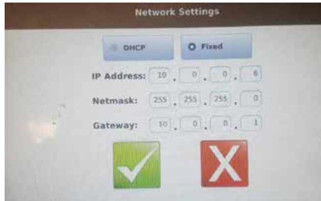
Figure 148: Changing the Internal IP Address (ST, QT, and N4 Models), Step 9
