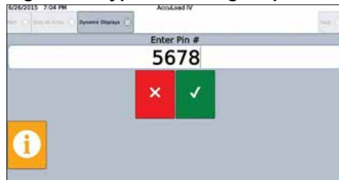
Figure 21: Typical Loading Sequence—Enter Pin Number, 2
