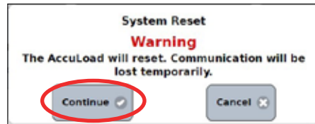
Figure 105: Resetting the System (Soft Restart), Step 3
