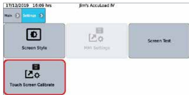
Figure 164: Main Menu, Device Settings, Touchscreen Calibration
