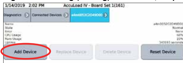
Figure 97: Adding (Pairing) I/O Boards, Step 3
