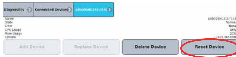
Figure 106: Resetting Individual I/O Boards (Soft Restart), Step 3
