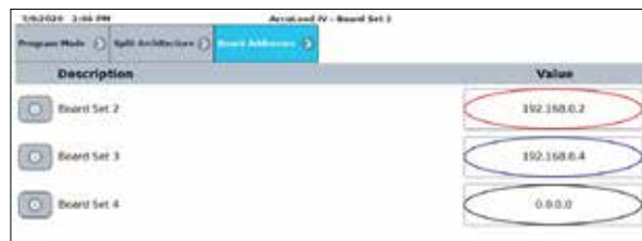
Figure 156: Changing the Internal IP Address (SA Model)—Board Set SAB
