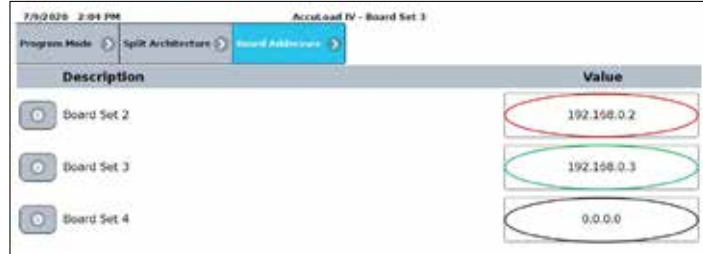
Figure 157: Changing the Internal IP Address (SA Model)—Board Set SAC
