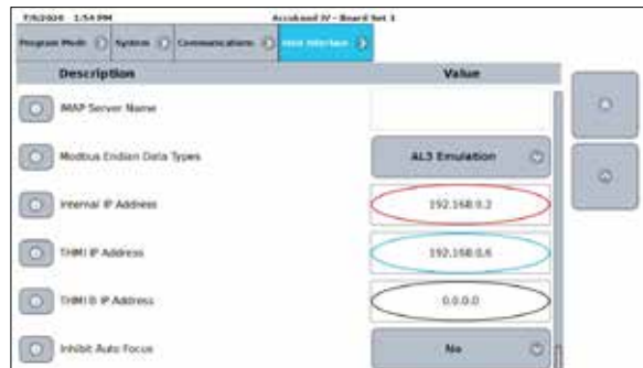
Figure 152: Changing the Internal IP Address (SA Model)—Board Set SAA
