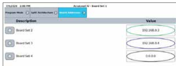
Figure 155: Changing the Internal IP Address (SA Model)—Board Set SAA
