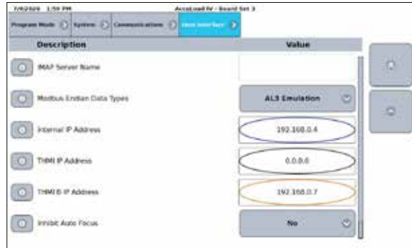
Figure 154: Changing the Internal IP Address (SA Model)—Board Set SAC
