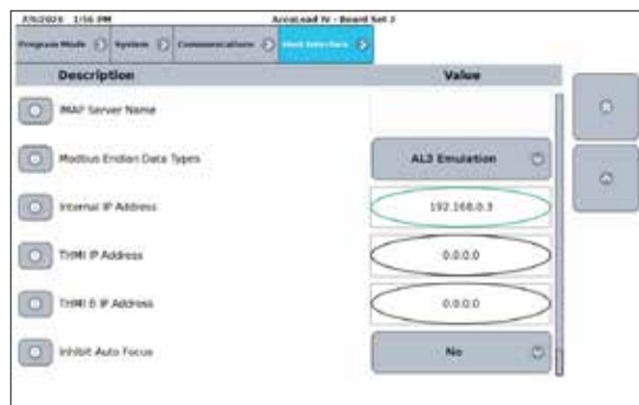
Figure 153: Changing the Internal IP Address (SA Model)—Board Set SAB
