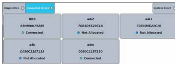
Figure 99: Adding (Pairing) I/O Boards, Step 5
