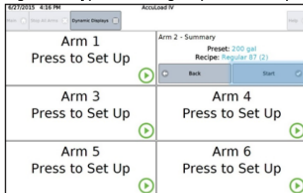
Figure 28: Typical Loading Sequence—Recipe Selection, 5
