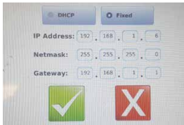
Figure 149: Changing the Internal IP Address (ST, QT, and N4 Models), Step 10
