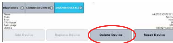
Figure 102: Deleting I/O Boards, Step 3
