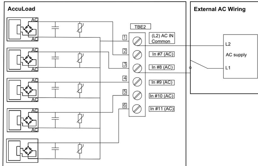
Figure 30: AC Digital Output
