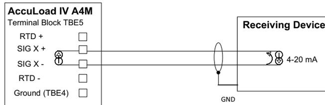
Figure 37: External Counter Wiring
