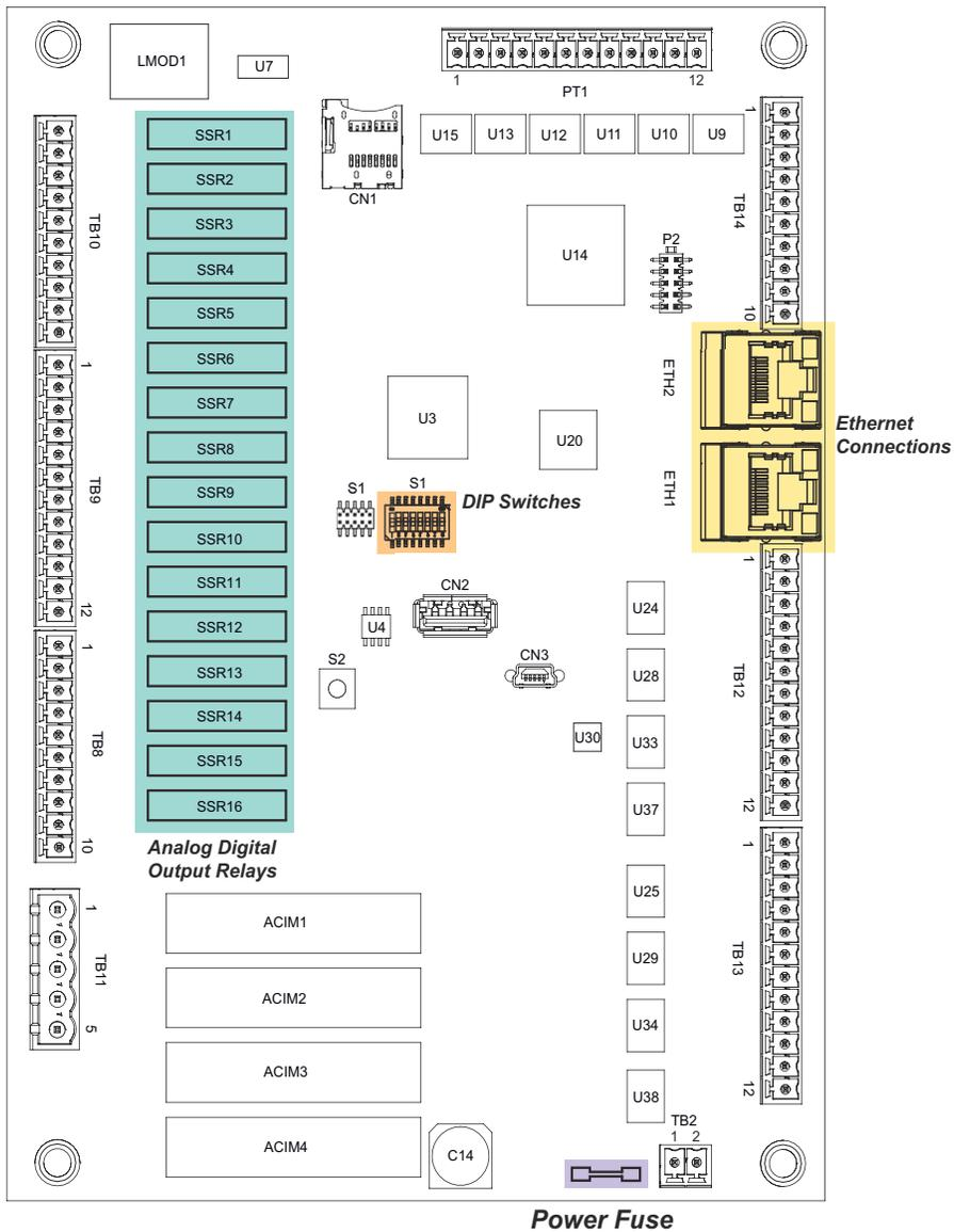
If digital valve control is used for any product- or flow-controlled additive meters connected to pulse inputs located on the A4M or A4B board, the digital outputs controlling the flow control valve must also be located on the A4M or A4B board, respectively.
