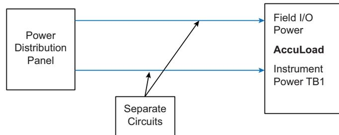
Figure 23: Example of AC Wiring for a Typical AccuLoad
