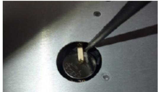
**Figure 58: Replacing the Battery**
