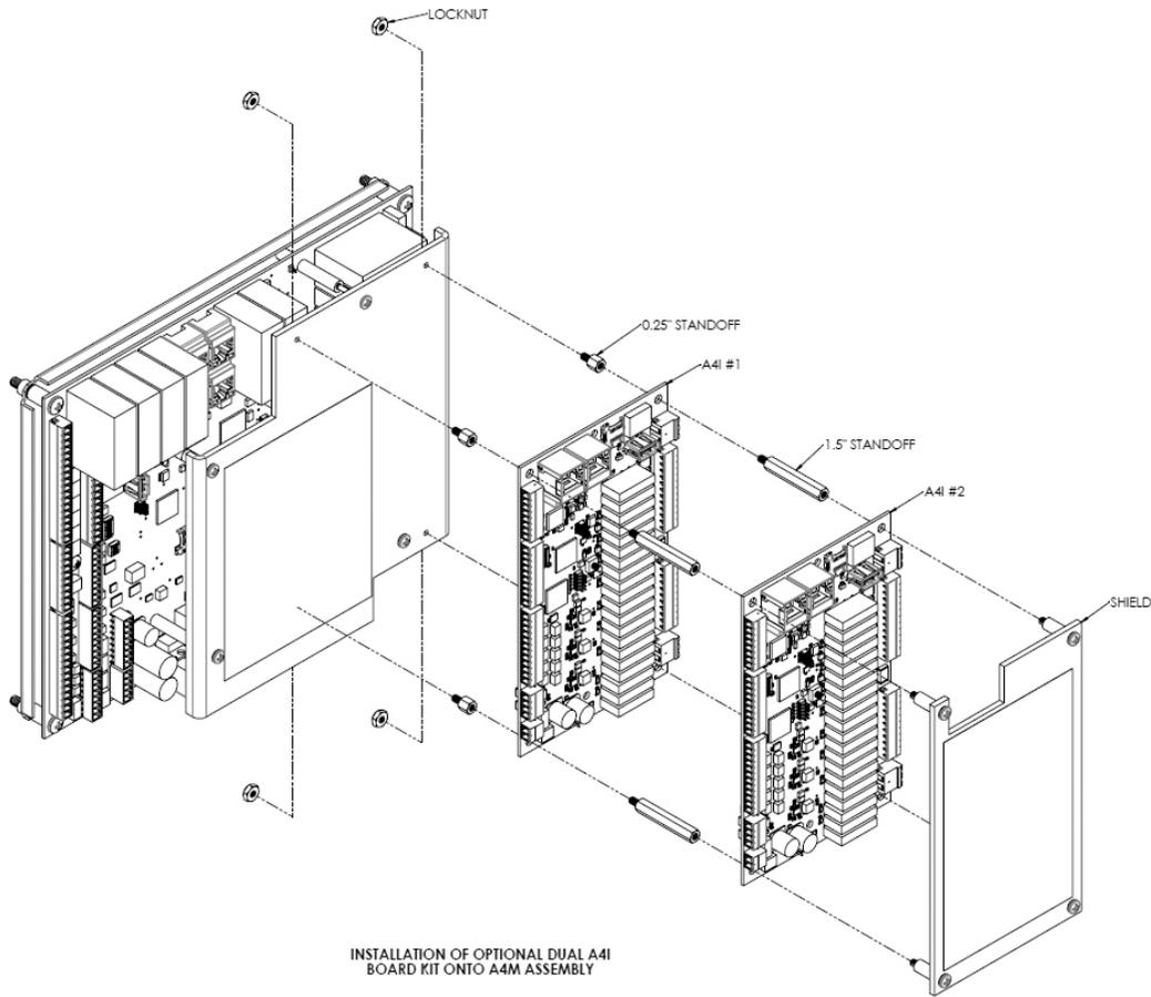
Complete the following steps to install one or two A4I boards onto the AccuLoad IV's A4M board:
