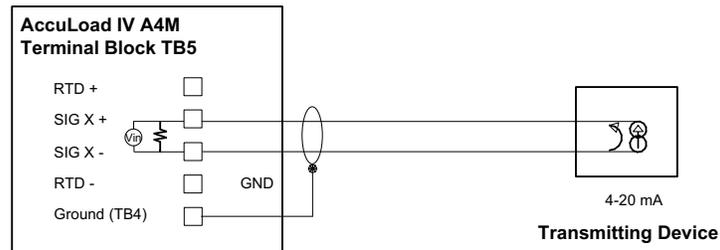
Figure 35: Passive 4-20 mA Analog Inputs
