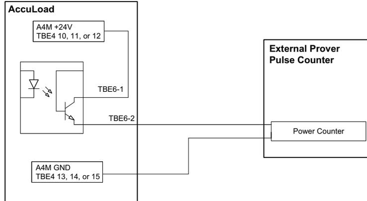
Figure 48: A4I Digital Input Wiring
