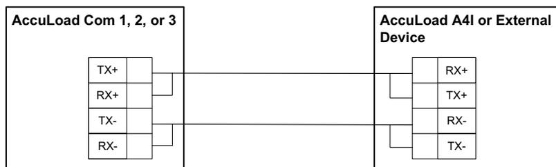
Figure 45: RS-232 Serial Wiring
