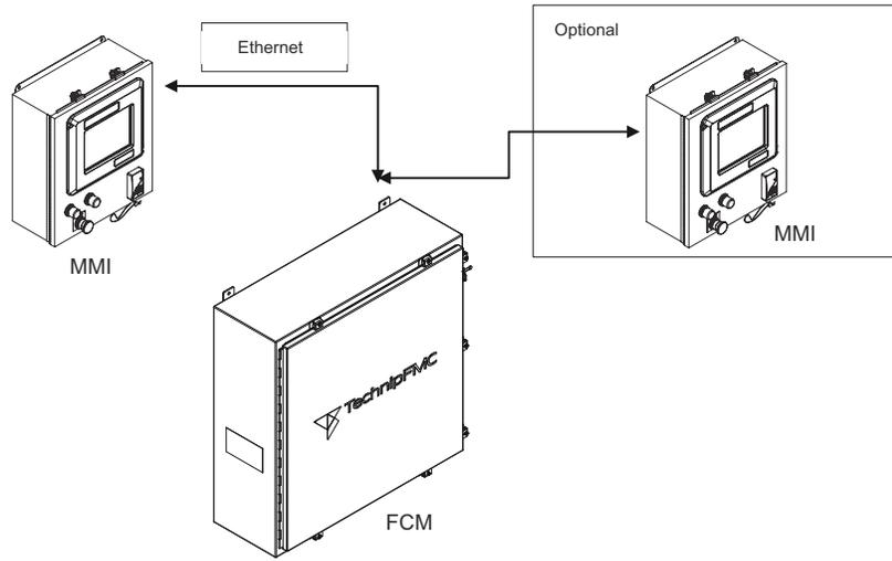
The FCM unit can be installed at a location that is convenient to service personnel. The MMI units can be installed for convenient access by drivers. Typical installation approaches are shown below.
