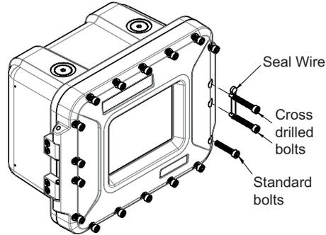
Figure 55: AccuLoad Model QT Sealing
