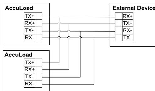
**Figure 44: Two-Wire RS-485 Serial Wiring**
