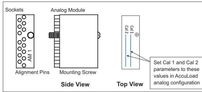
**CAUTION:** Before inserting or removing any analog module, first ensure that all associated circuits are de-energized. Use proper ESD practices. To remove a module, loosen the captive retaining screw and then gently pull the module out of the socket while slightly rocking the module.
