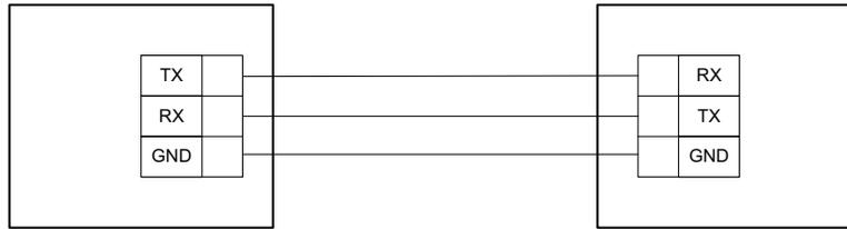
Figure 46: Multi-Drop RS-232 Serial Wiring
