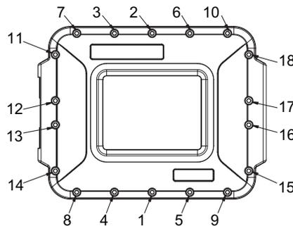
**Figure 52: Cover Bolt Torque Pattern for AccuLoad IV Model QT**
