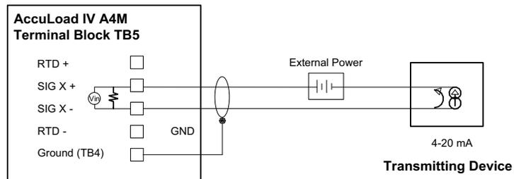
Figure 36: Analog Outputs
