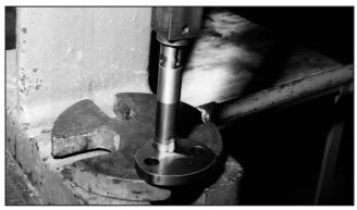
Figure 14 – Press Shaft into Cam
