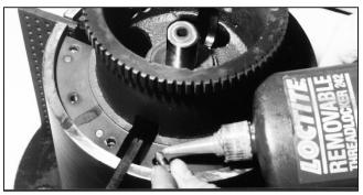
Figure 16 – Replace Rotor Cover
