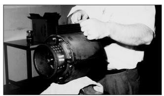
*Figure 21 – File Blade to Increase Blade Tip Clearance* Repeat as necessary until all blade tip clearances are between 0.0025" and 0.0045".
