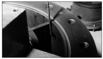
Figure 20 – Measure Blade Tip Clearance
