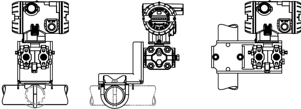
**Figure 2 — Examples of typical mounting positions (antenna omitted)**
