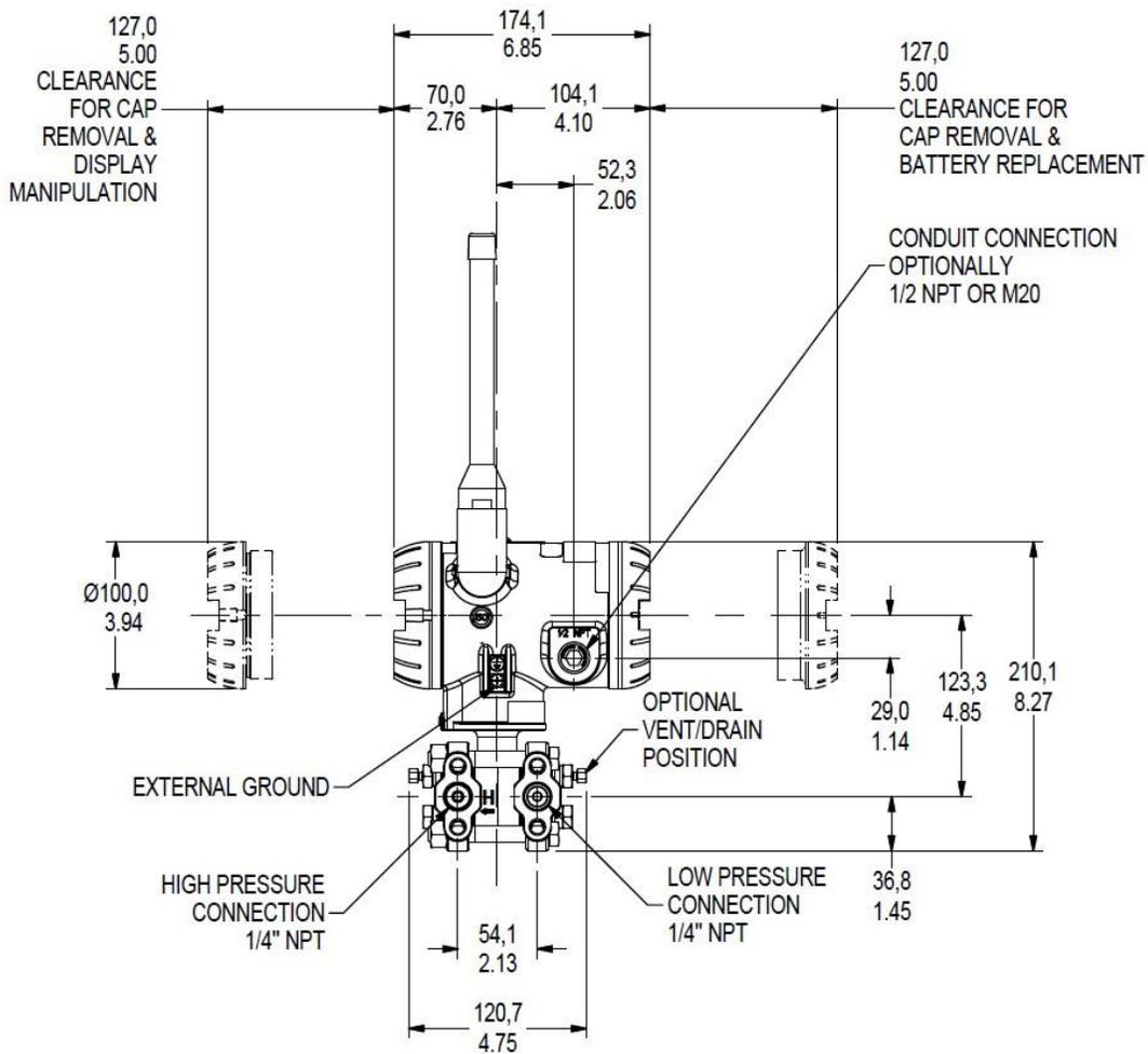
**Figure 3 – Informational and dimensional drawing (4 dBi antenna shown)**
