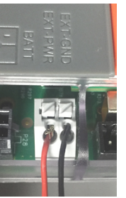
6 Connect power supply wires from the terminal box
