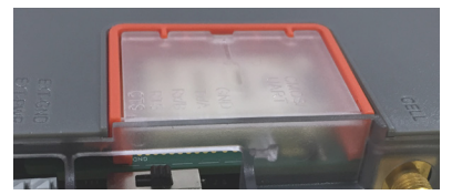
1 Remove the SIM card cover and insert the SIM card
