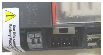
4 Connect to external power supply or battery power 4.8V to 30V, External power supply.
