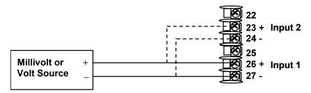
Table 6-7: Set Up Wiring Procedure for Millivolts, Volts or Thermocouple Differential Inputs
