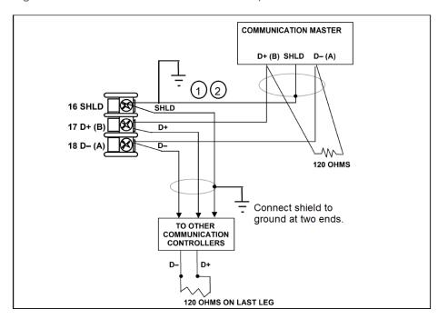
Figure 3-13: RS485 Communications Option Connections
