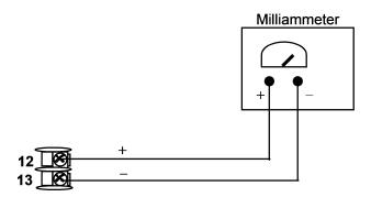
Table 7-3: Set Up Wiring Procedure for Auxiliary Output
