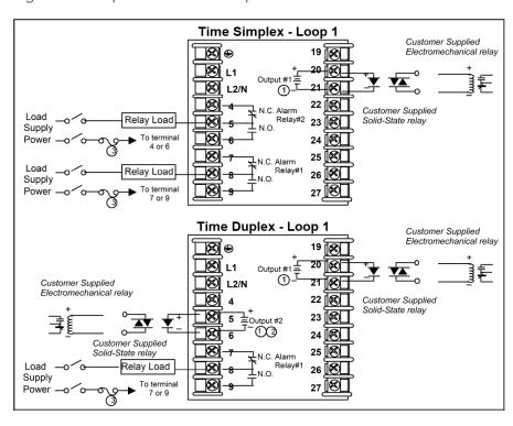
Figure 3-8: Open Collector Output
