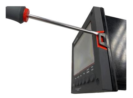
Using a thin screwdriver, gently twist the screwdriver to pry the side tabs from the front face. Pry just enough to release it, otherwise you'll bend or break the tab. If you break or bend the tab and can't reattach the front snugly, you'll need to reattach the front using the 4 NEMA4 screws provided. See Mounting for more information.
