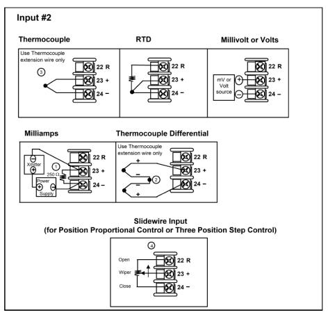
Figure 3-6: Input 2 Connections
