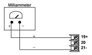
Table 7-1: Set Up Wiring Procedure for Current Output
