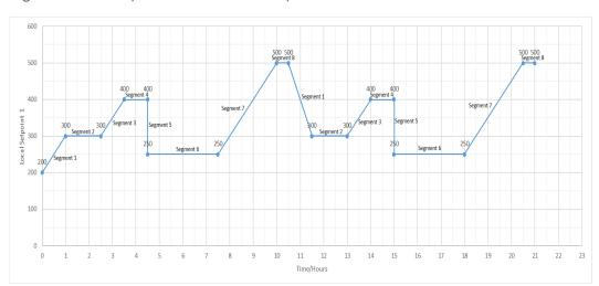
Figure 5-7: Ramp/Soak Profile Example
