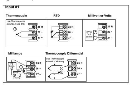
Figure 3-5: Input 1 Connections
