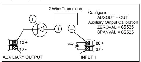
Figure 3-17: Transmitter Power for 4-20 mA - 2 Wire Transmitter Using Auxiliary Output
